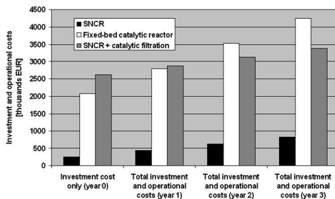
Fig. 12. Investment and operational costs calculated for three different deNOx technologies for a MSW incineration plant with flue gas production of 65,000  $\text{N m}^3/\text{h}$  and input NOx concentration of 550  $\text{mg}/\text{N m}^3$  (costs calculations based on European IPPC Bureau, 2008a).
