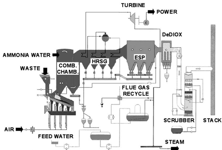
Fig. 2. Scheme of MSW incineration plant with installed catalytic filter.
