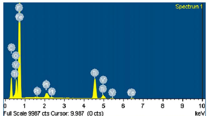
Fig. 9. Result of analysis of filtration bag after water extraction (diagram reveals no presence of sulphur compounds (S), calcium compounds (K) and sodium compounds (Na)).
