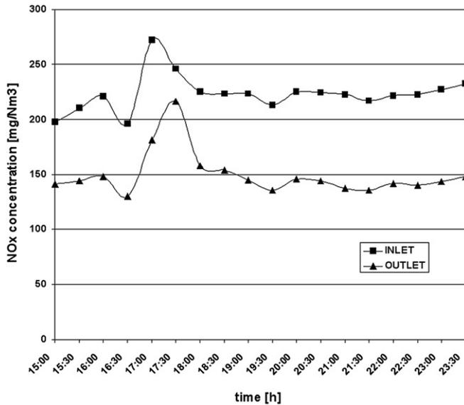
Fig. 6. Standard measured efficiency of new filtration bags in reduction of NO<sub>x</sub>; average temperature of 228 °C, molar ratio NH<sub>3</sub>:NO = 1.1 mol/mol, average NO<sub>x</sub> disposal efficiency equaled 33.2%, dry flue gas, concentration recalculated for reference oxygen O<sub>2</sub> = 11%.
