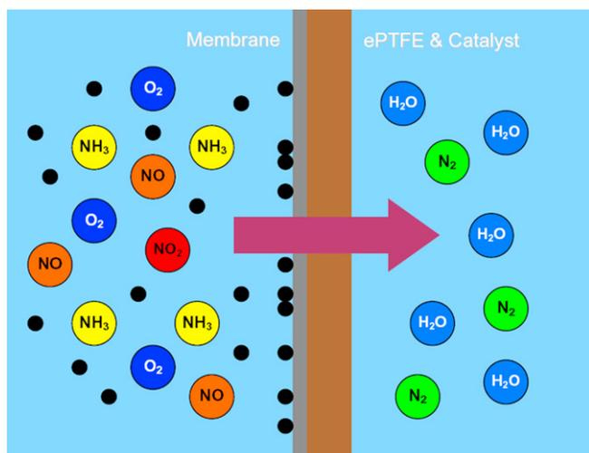
Fig. 3. Principle of decomposition of NO<sub>x</sub> at catalytic filter.
