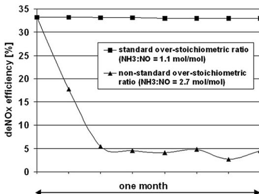
Fig. 7. Comparison of long-term deNO<sub>x</sub> efficiency for standard and nonstandard conditions.
