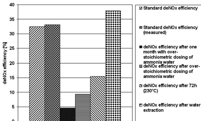
Fig. 10. Overview of new filtration bag efficiencies during individual phases of operations and testing.
