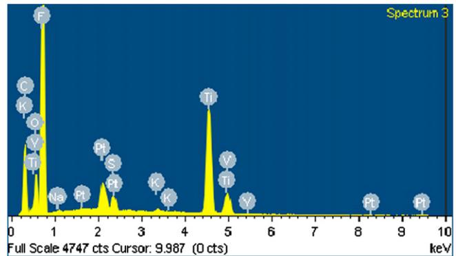
Fig. 8. Result of filtration bag analysis (diagram presents high amount of sulphur compounds (S), calcium compounds (K) and sodium compounds (Na)).
