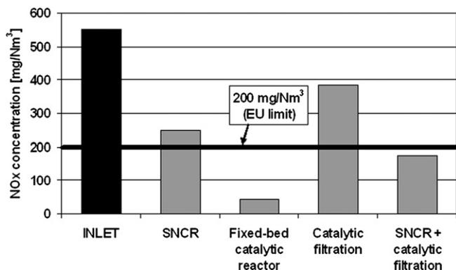
Fig. 11. Example of potential decrease of NOx concentration in flue gas by application of various methods.
